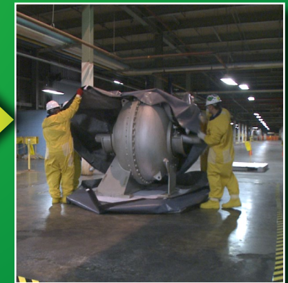
The compressor is secured in a soft-sided shipping container for storage prior to shipment.
